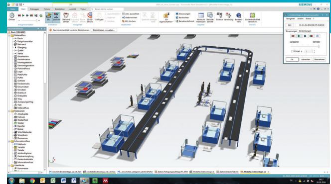
Building the digital twin of the radiator production line allowed the WP manufacturing engineers to include worker-related actions.
