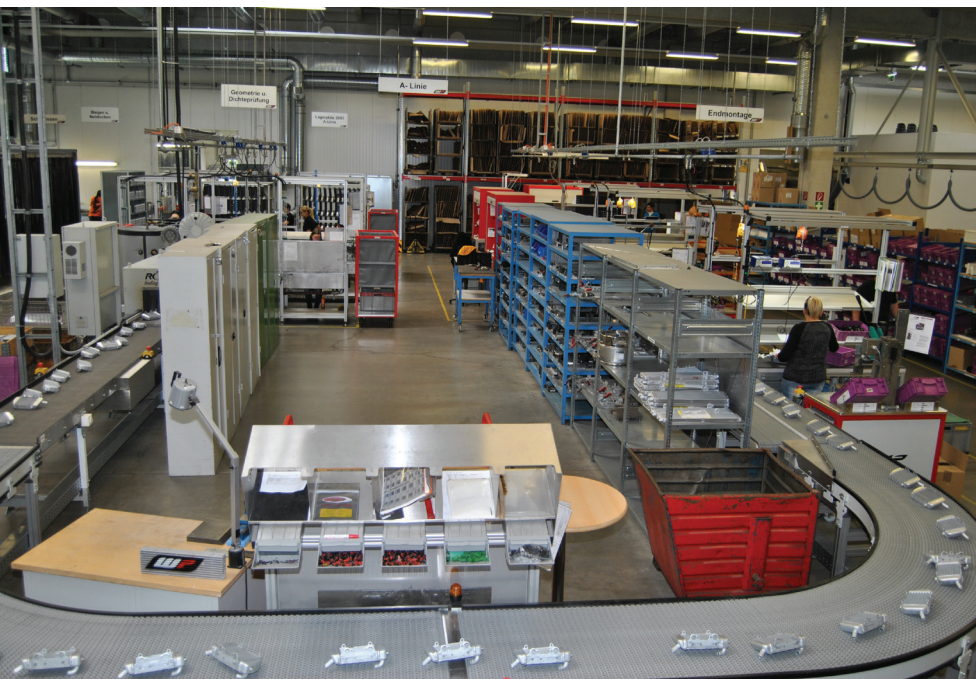
Separating the A parts from the lower quantity varieties and building them in a cyclic flow production along a U-shaped conveyor allowed WP Components to increase output by 40 percent without requiring more room or extra workers.
