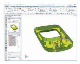
ibility of the designs, increase the operational life of the part and reduce manufacturing costs. Some of the important rules supported for castings checks include fillet radius, surface finish for machined faces, uniform wall thickness, mold wall thickness, wall thickness variation, draft angle and undercut detection.
