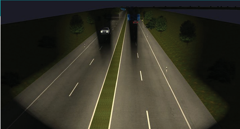
The LED Matrix headlight automatically masks oncoming or leading vehicles while brightly illuminating their surroundings. Photo: ZKW.
