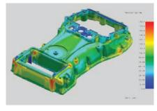
the given design and process conditions. This is the time estimated from cooling analysis for the computed mold cavity surface temperature, and the estimated center temperature of the plastic part to be cooled enough to be ejected. This value can be used as an indicator of hot spot and cycle time-restriction locations.
